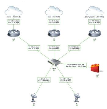
The NOC uses Zabbix to monitor all active equipment deployed into various areas of the venue. The tool enables the NOC to respond quickly to power outages, network problems, and equipment failures. The NOC is where the Meetings, Meetings Technical Services, and Security teams work together to ensure quick inter-departmental communications and coordination.
